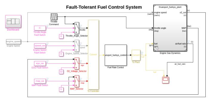
Open the Dashboard subsystem to simulate any combination of sensor failures.
