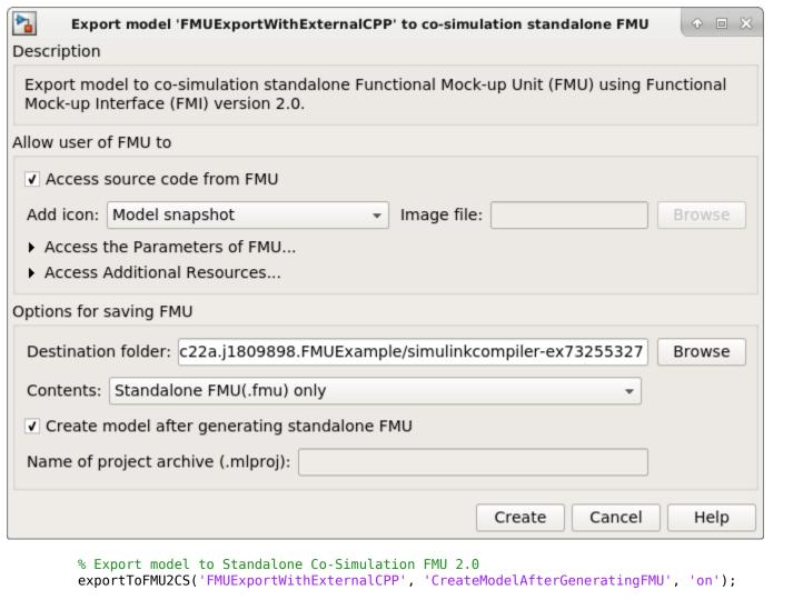
Setting System Target to FMU Co-Simulation for model 'FMUExportWithExternalCPP'.
