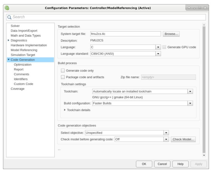
% alternative command-line option to set protected model code generation target to fmu2cs.tlc % this allows the protected model to be exported as standalone FMU set\_param(model, 'SystemTargetFile', 'fmu2cs.tlc');
